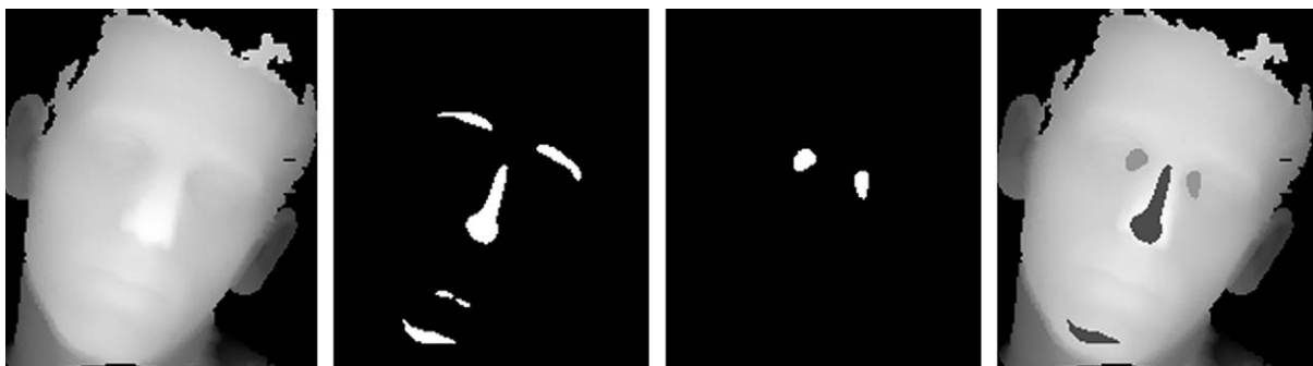
Fig. 4. From left to right: a range image generated by an orthographic projection of a polygonal model; the image used to localize nose candidates; the image used to localize eye candidates; the regions selected for generation of the face triangle.
