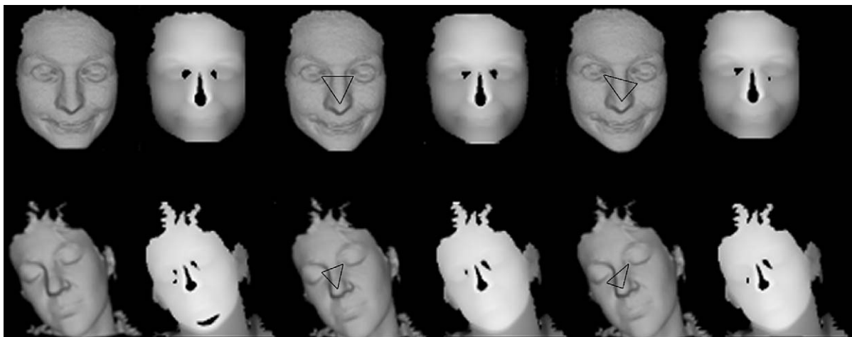
Fig. 13. Two examples of the overlapping face triangle problem. As can be seen, in each case a small candidate eye is generated near the true eyes; as a consequence more than one candidate face is generated for the same real face.
