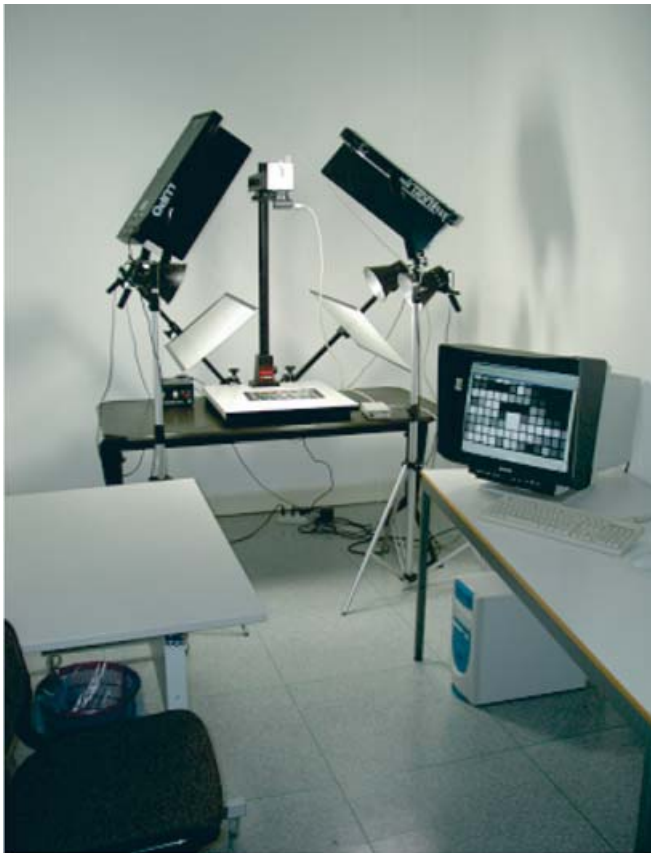
Fig. 2. Wideband multispectral acquisition systems can be mounted on a tripod but also hanged from above using a simple frame like this one
