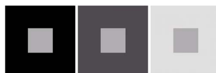
FIGURE 2.8 Examples of simultaneous contrast. All the inner squares have the same intensity, but they appear progressively darker as the background becomes lighter.
